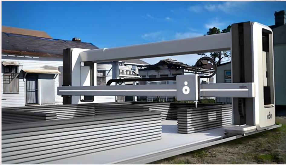
Figure: ICON VULCAN 2 – Used for 3D printing houses using concrete extrusion
