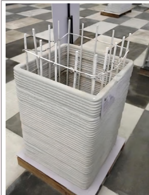
Figure: The concrete mould printed
