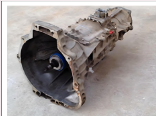
Figure: Manual transmission for a four-wheel-drive vehicle (Ford Ranger) viewed from the engine side
