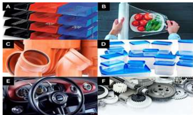
Different types of polymer materials and their applications (A) high-impact polystyrene (HIPS)—stationery trays; (B) polyvinyl alcohol (PVA)—food wrap; (C) acrylonitrile styrene acrylate (ASA)—drain pipes and fittings; (D) polypropylene (PP)—food containers; (E) polycarbonate ABS alloy (PC-ABS)—glove box; (F) gears.
